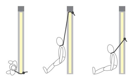
Ligature points can be both high and low. The loading pattern will differ depending on the anchor point height and direction of body lean/fall.
